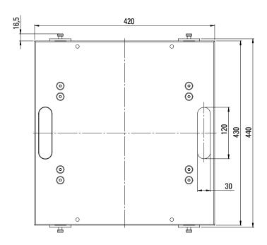
Weighing area L 430 mm x W 420 mm Height 30 mm
