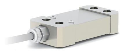
For strains up to  $\pm 750\,\mu\text{E}$  CANopen signal output Optional with integrated measuring amplifier with analogue current and voltage output Encased design IP 67
